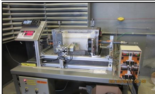
On-line laser creep test
